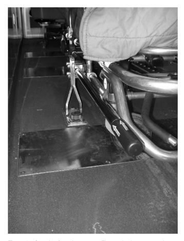
$\label{eq:Figure 3} \mbox{ Stretcher-fastening system. The mechanism secures the stretcher to the ambulance floor during transportation.}$
