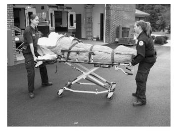
**Figure 1** Adjusting ambulance stretcher height. Ambulance personnel must simultaneously activate mechanical triggers at each end of the stretcher, coordinate manual stretcher lifting or lowering, then re-actuate the mechanism to lock the wheeled undercarriage in place.
