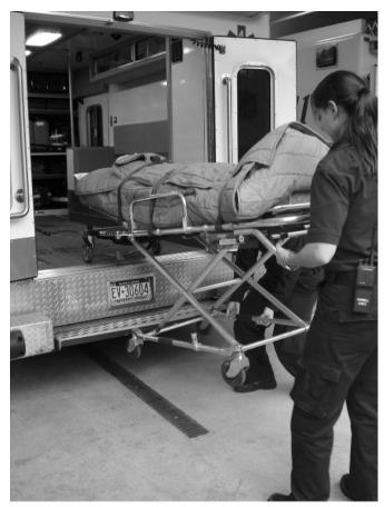
**Figure 2** Unloading stretcher from ambulance. One operator lifts the foot of the stretcher out of the ambulance while the other operators guides the wheeled undercarriage until it locks in place. A safety catch bar prevents the head of the stretcher from rolling out of the ambulance.
